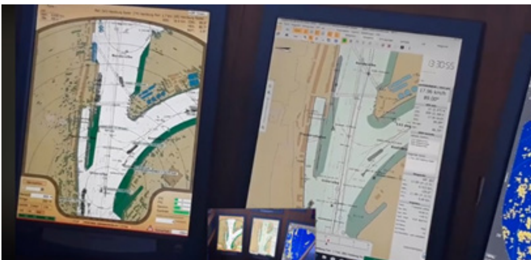
Figure 4 Periskal Radar Overlay /Periskal IE Viewer with Argonics interface
